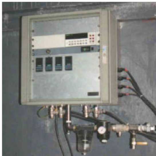
Figure 3: View of the VTER instrumentation and probe cooling system.
