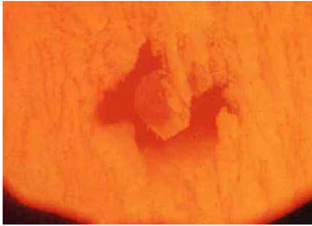
Figure 4: VTER furnace wall corrosion probe installed in the wall of a combustor.
