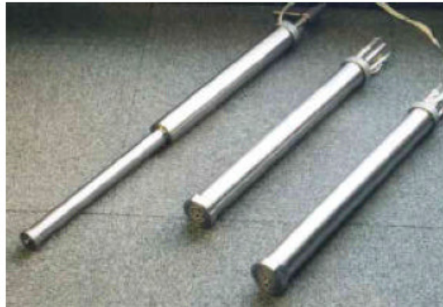
Figure 2: VTER superheater and furnace wall corrosion probes.
